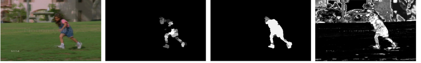
Fig. 4. Positive predictions of each region and the brightness indicates probability of being an object: (a) source image; (b) independent SVM predictions; (c) predictions from graph transduction capturing the coherent intrinsic structure within visual data, using SVM predictions as input; (d) per-pixel object probabilities from GMM color model trained using object proposals.
